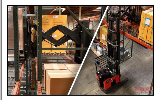
**Double deep reach trucks** have double extended reach so the operator can reach deeper into racking.
