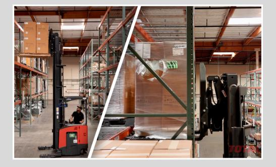
**Single reach trucks** can reach into 1 pallet deep racks, allowing unobstructed access to each pallet.
