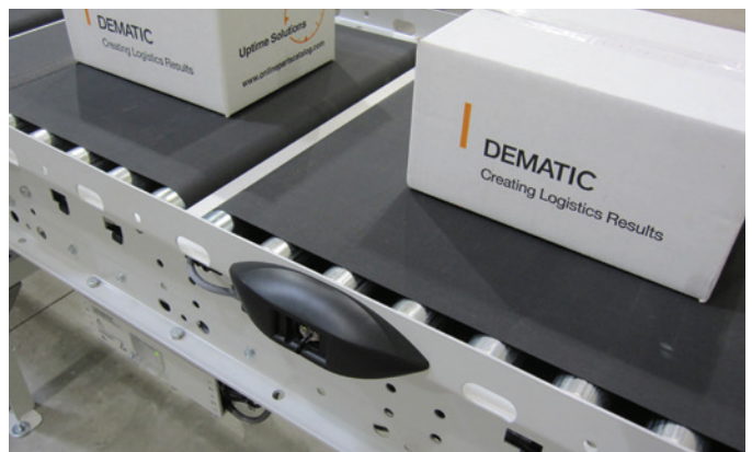
Cover on side channel protects electronic sensor
