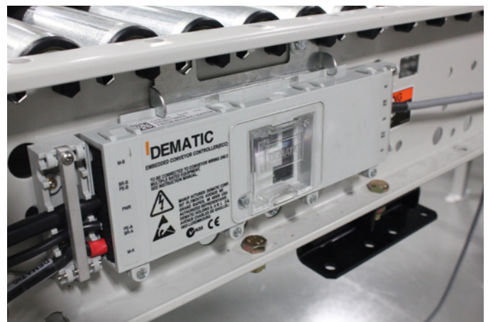
Embedded Conveyor Controller (ECC) controls the operation of motorized roller conveyor
