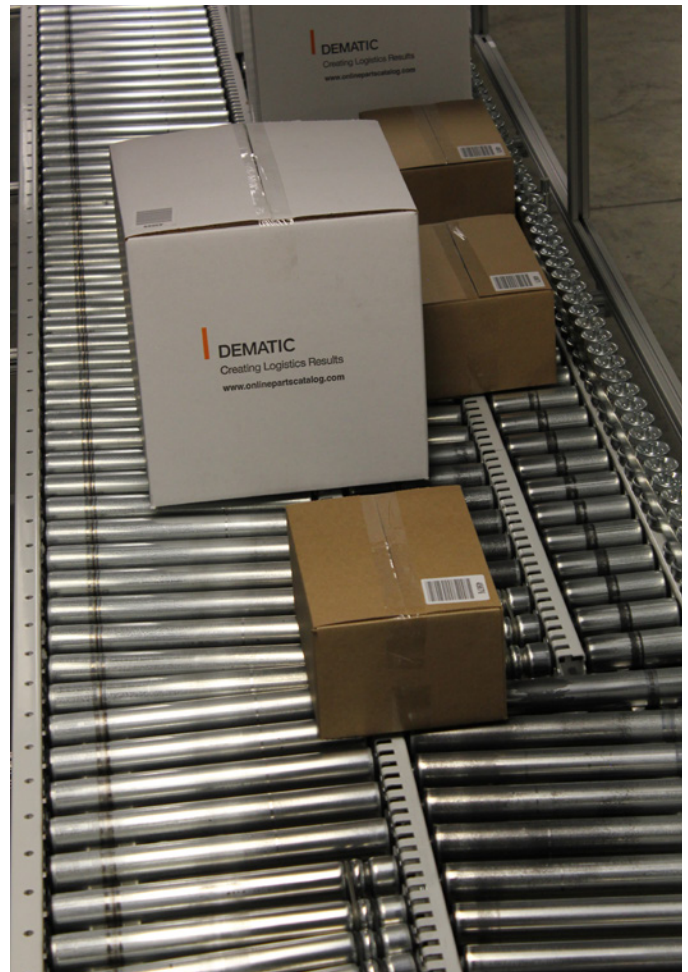
The singulator improves downstream merge and sorter performance
