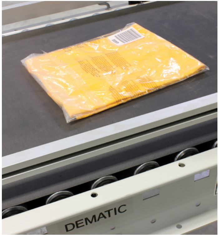
Segmented belt on roller accommodates apparel in poly bag
