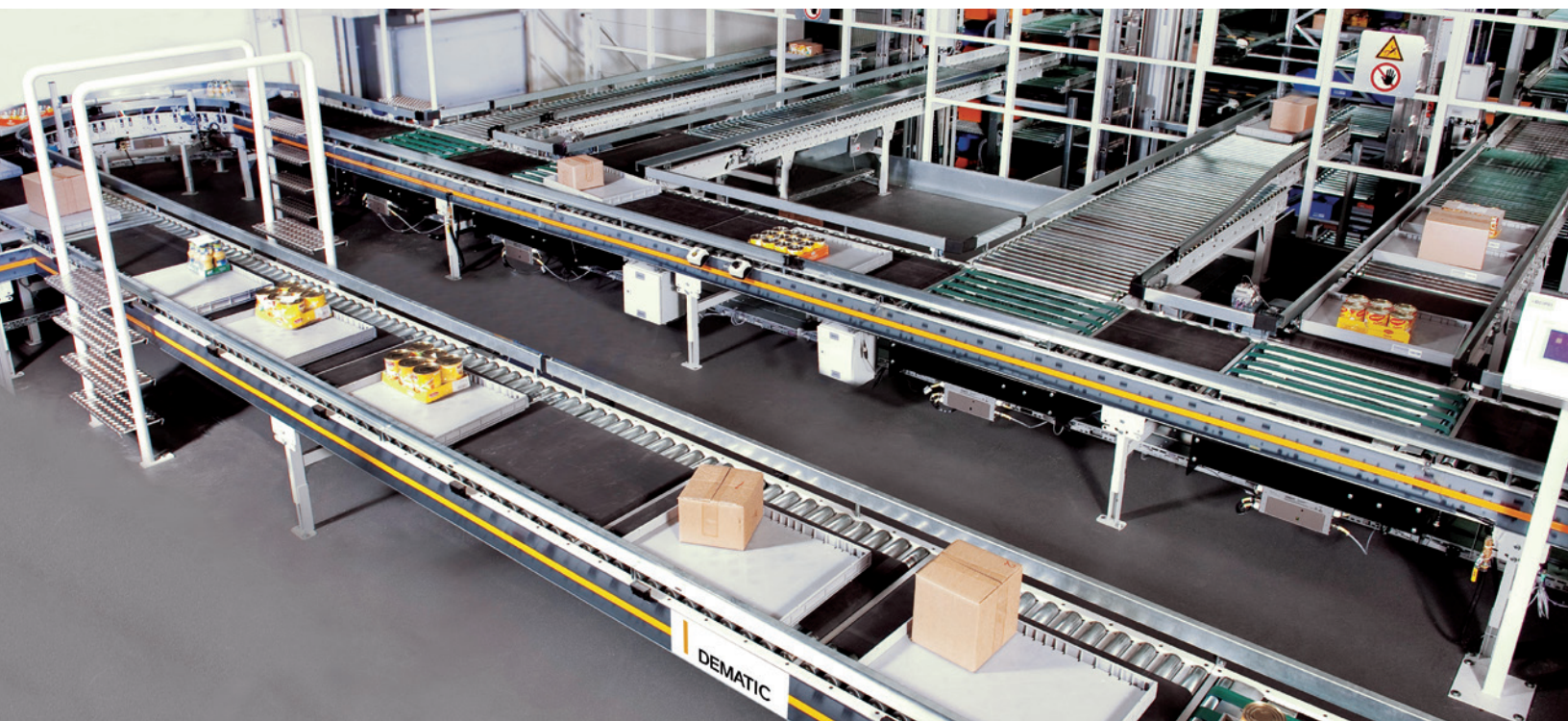
Accumulating conveyor with electronic sensing
